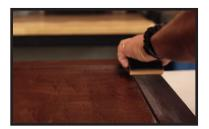
**PRO TIP:** When sanding, move the sandpaper in the same direction of the wood grain. If you go against the grain you will end up with a lot of nasty scratches that will show through your topcoat.
